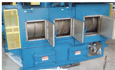
Close up of Rotary Drum (left). Combination Rotary Drum and Flat Belt Conveyor Washer for Aqueous Degreasing (above). A Monorail and Rotary Drum washer is also available.
