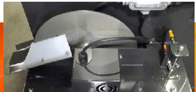
Oil Skimmer and Tank Low Level Switch
