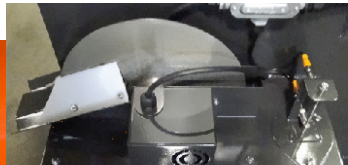
Oil Skimmer and Tank Low Level Switch
